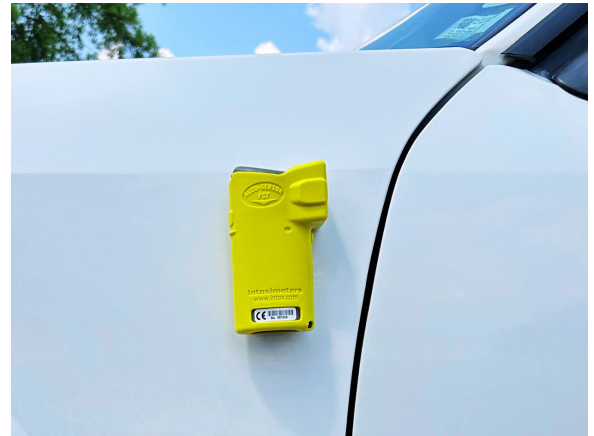
Bilateral magnets on outer sides of the instrument securely attach to ferrous metal surfaces.
